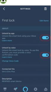
Enable unlocking by App or Voice as shown above. For Activation by app: You must turn on the Unlock by App option and put in your Amazon Alexa app password to enable it. For Activation by Voice: You must turn on the Unlock by voice option and enter your
