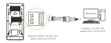
Click [COMM.] > [Ethernet] > [IP Address], input the IP address and click [OK].
