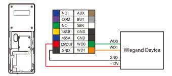
**Note:** The Wiegand interface is shared, and the user can choose to use either the Wiegand input or Wiegand output function to interface with different Wiegand devices.
