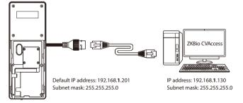
Tap on  $\blacksquare$  to enter the main menu. And then click on [Comm.] > [Ethernet] > [IP Address] to input the IP address.
